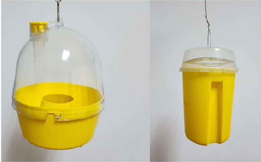
Figure 1: Medfly trap designs used in (left) Costa Rica (McPhail traps) and (right) Tunisia (Tephriti traps) to capture Ceratitidis capitata .
